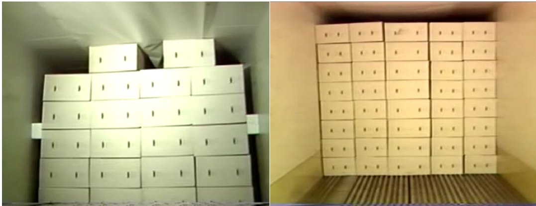
Left: loaded too high, right: loaded too wide
