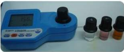
Colorimetric equipment for measuring concentration of free chlorine in the washing water.
